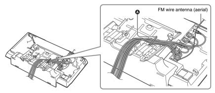
Thread the AC power cord (mains lead) through the gap on the main unit by securing it behind the tabs, guide it through the slot at the left of the main unit, behind the clamp (3), and through the slot at the bottom of the main unit.
